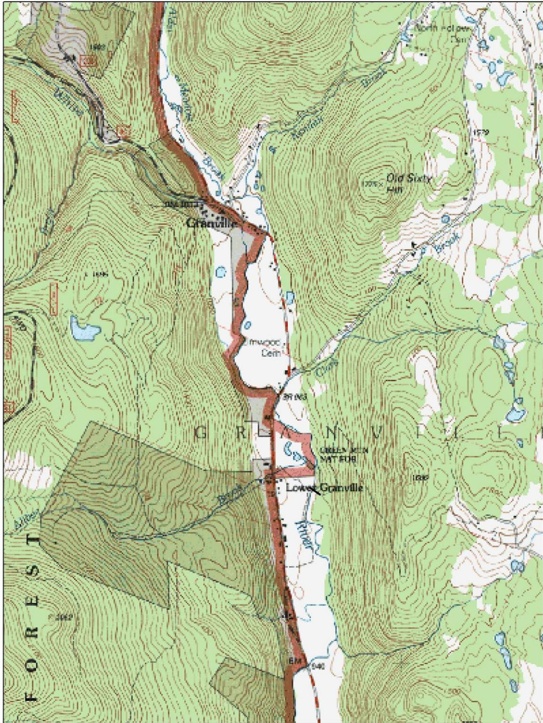
Figure 19. Although no alluvial fans were identified in Phase 1 or Phase 2 assessment of the Upper White, the confluence of several streams at the base of steep valley walls in a relatively narrow valley setting suggest that the presence of a combined fan, or several fans, may be masked by development and agricultural lands in the upstream portion of reach R24 and reach R25 near Lower Granville and Granville.
