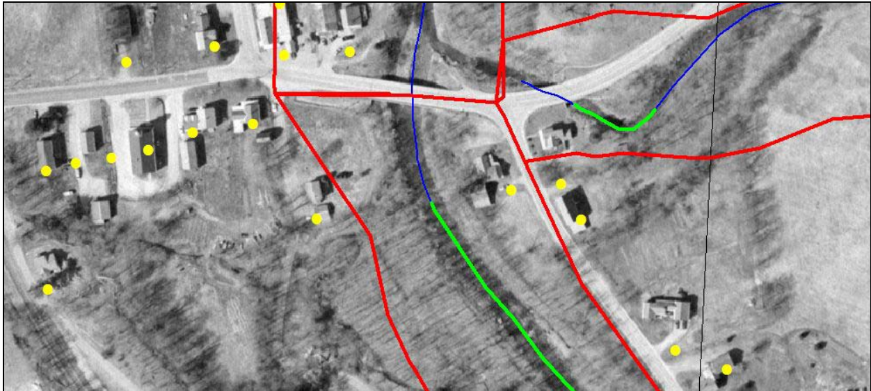
Figure 2: FEH Zone (red), berms (green) and structures at end of reaches M11-A and T2.01-A.
