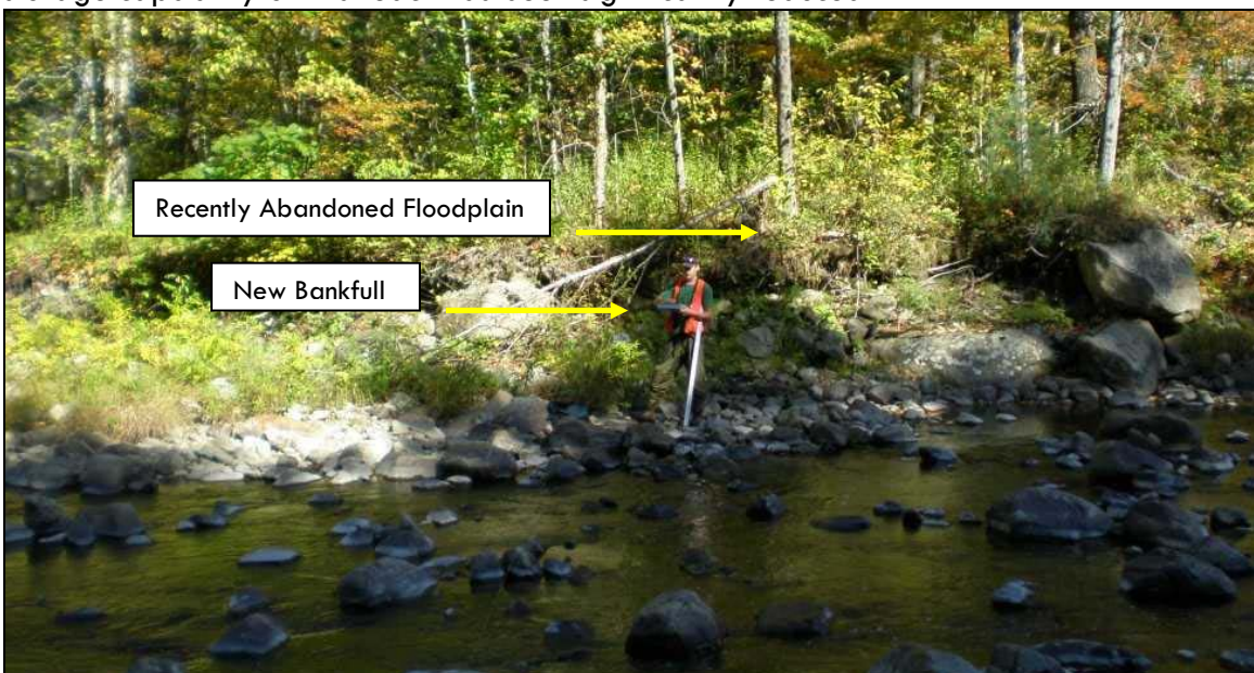
Figure 14. M08 is a short reach that has limited floodplain access due to streambed degradation.
