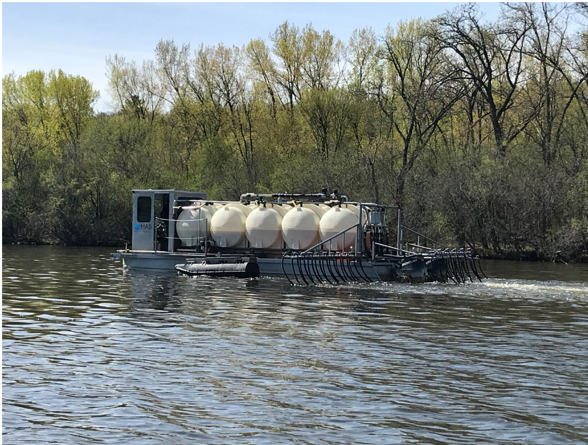
Figure 1 Example of a barge used to apply alum and sodium aluminate.
