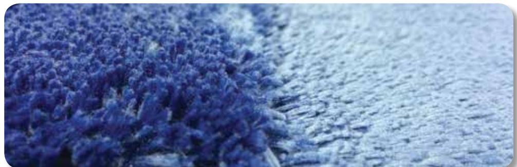
Shown is pile cloth media in its natural state (left) and its conditioned state (right).
