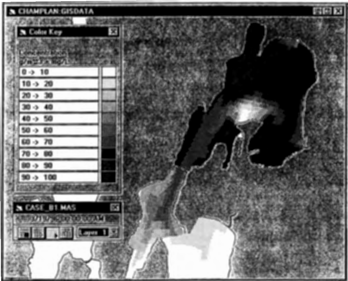
Figure 6.25(a) Plan view of vertically averaged water column concentrations for Case B1 (base case with present causeway configuration).
