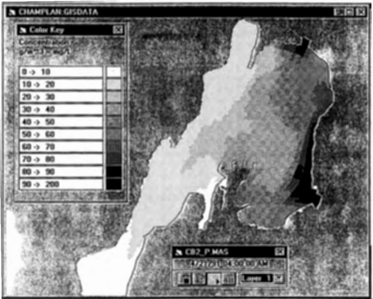
Figure 6.46 Plan view of vertically averaged water column phosphorus concentration for Case B2 (base case with the causeway completely removed).
