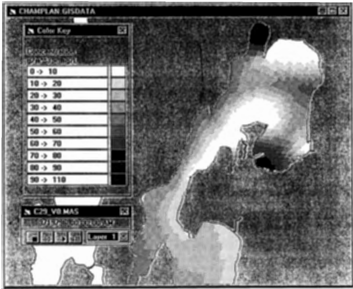
Figure 6.34 Plan view of vertically averaged water column concentrations for Case 29 (no wind with causeway completely removed).
