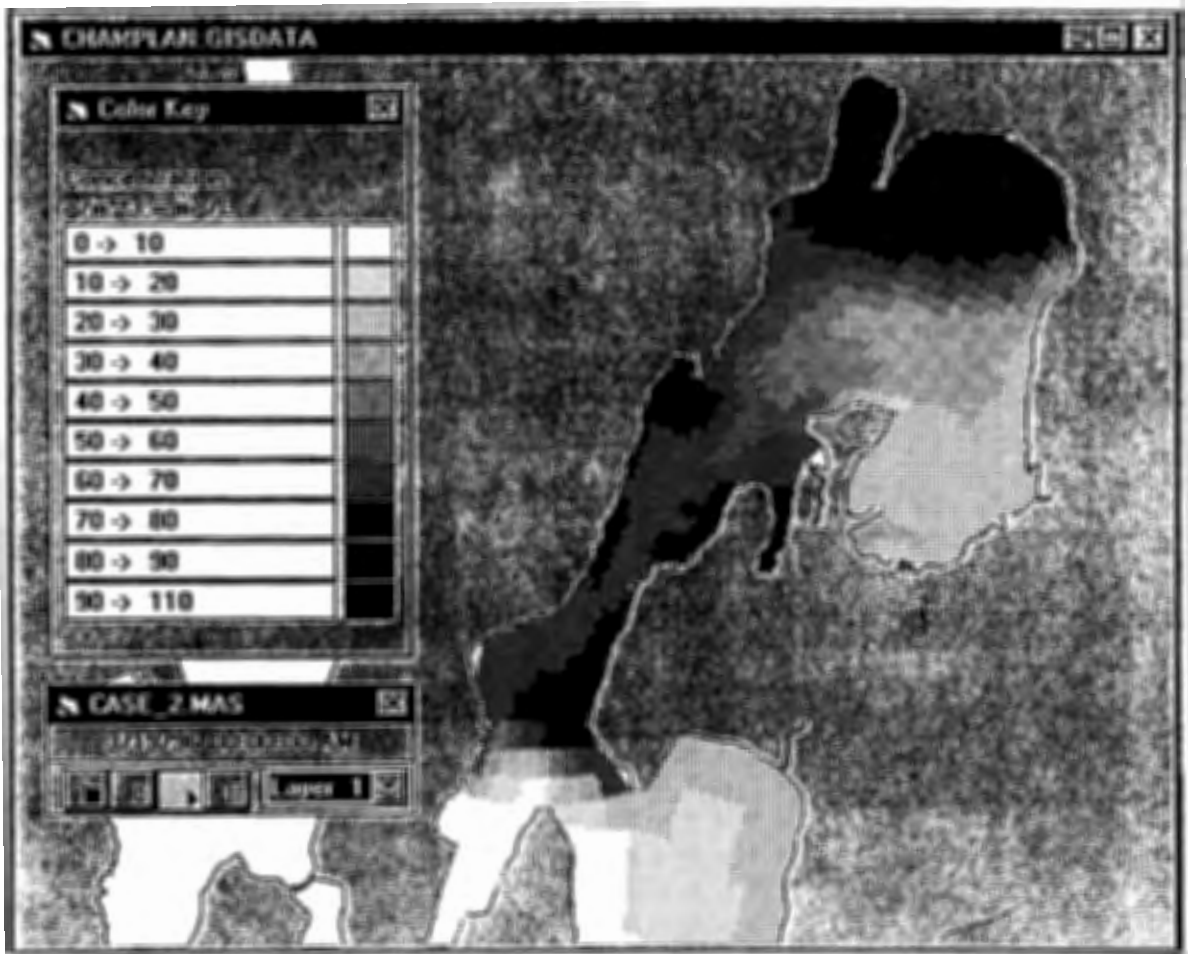
Figure 6.28 Plan view of vertically averaged water column concentrations for Case 2 (west wind with the causeway completely removed).
