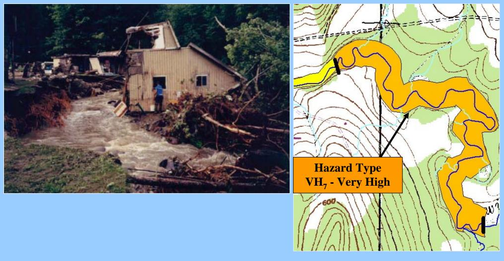
Uses geomorphic assessment data to mitigate flood-related erosion hazards by identifying, mapping and protecting river corridors
