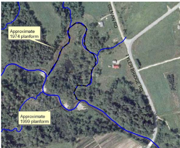
Figure 12. Abandoned meander at mid-section of reach M15 (Segment B) downstream of the Tyler Bridge Rd bridge. Review of annual fly-over images at the NRCS Middlebury office indicates that this avulsion occurred over a period of time from 1994 to 1995. Cut off of this broad meander resulted in a loss of 1000 ft of channel length. The avulsion and subsequent channel adjustments may have contributed to recent aggradation in Segment A. (Base image is dated 2003)
