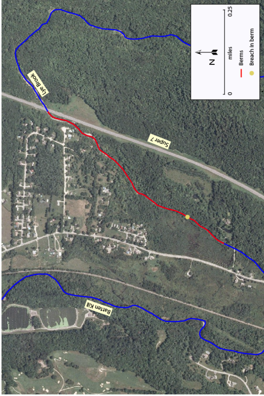
Figure 16. Close up of Lye Brook alluvial fan showing location of berms relative to human developments.
