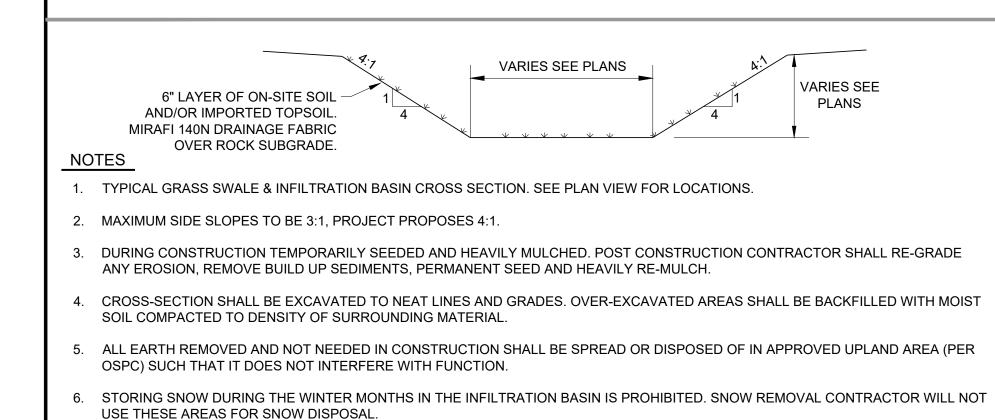
GRASS SWALE & INFILTRATION BASIN CROSS SECTION N.T.S. DISCONNECTION FOR CONTRIBUTING IMPERVIOUS SURFACE, GRADE CONTRIBUTING IMPERVIOUS SURFACES TO DRAIN WITHOUT CONCENTRATING FLOWS. SEE DETAIL FOR SUBBASE SPECIFICATIONS.
