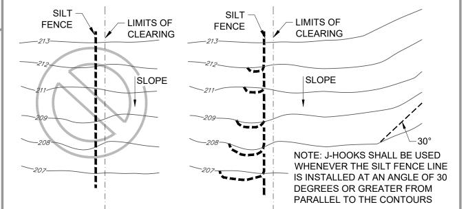
**INCORRECT** SILT FENCE INSTALLED PARALLEL TO SLOPE (PERPENDICULAR TO CONTOUR) IN ONE, LONG RUN
