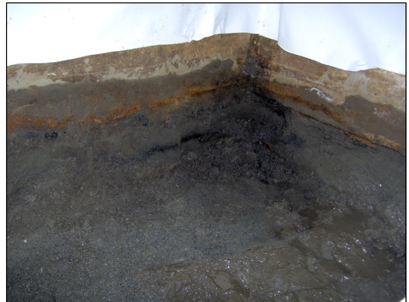
Photo #4: Dark staining against SE corner, likely related to contamination
