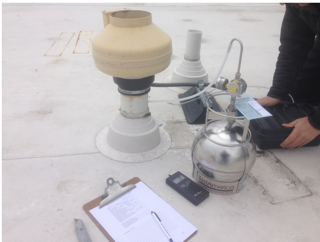
Photograph of the air sample collection apparatus
