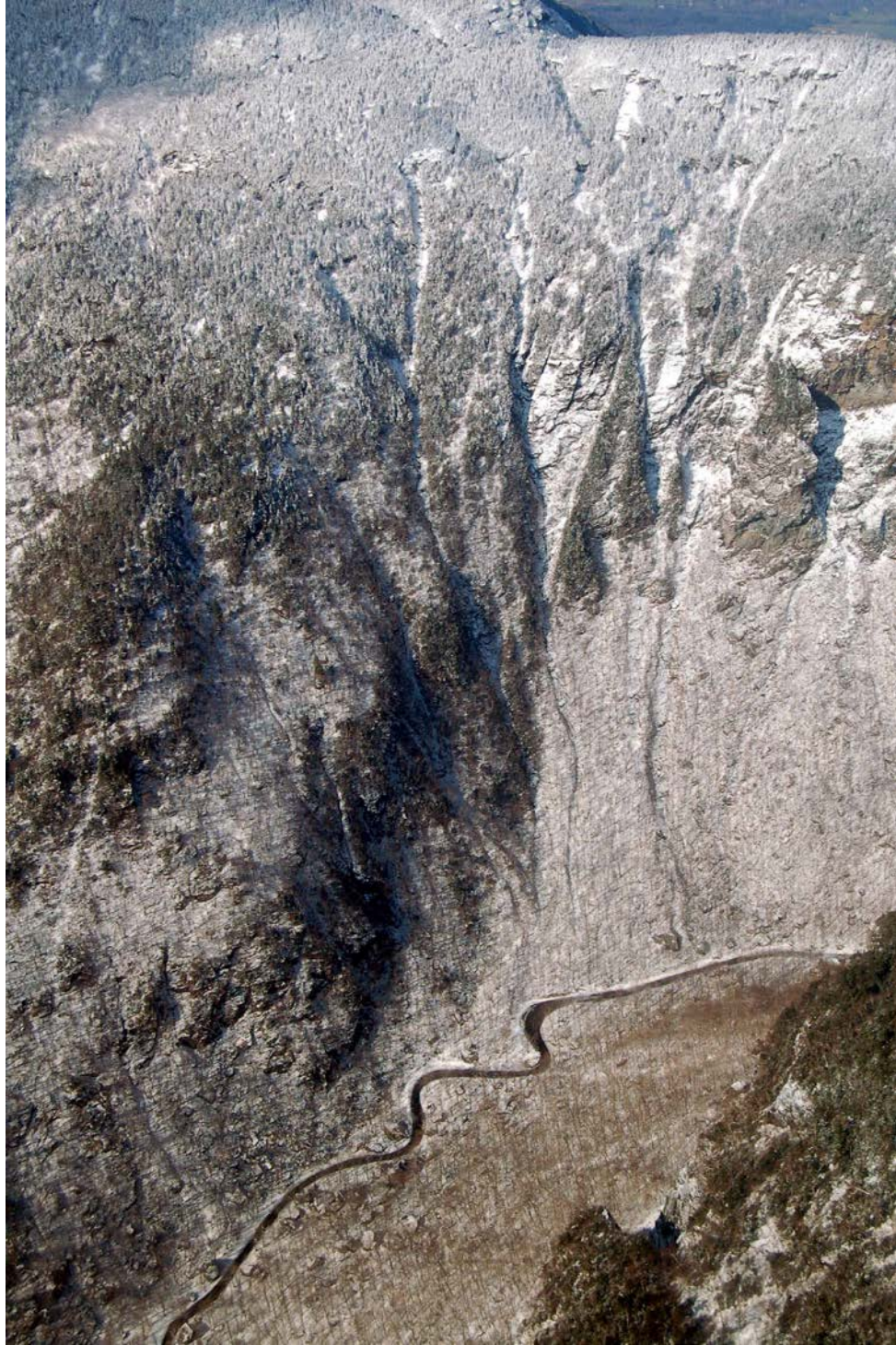
Figure 4.9. Aerial view of the western cliffs and debris flow tracks south of Cass's Gully. Note that the rock chutes that feed some of the tracks extend up above the main cliffs almost up to the ridgeline. Photograph taken on November 9, 2007 by Tom Eliassen, Vermont Agency of Transportation.
