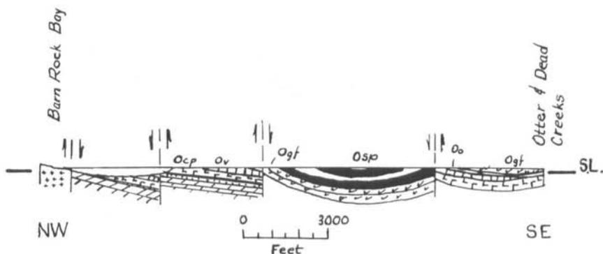
Text-fig. 18. Diagrammatic cross-section from Barn Rock Bay, N.Y., to juncture of Otter Creek and Dead Creek, Ferrisburg, to show horst and graben structure.
