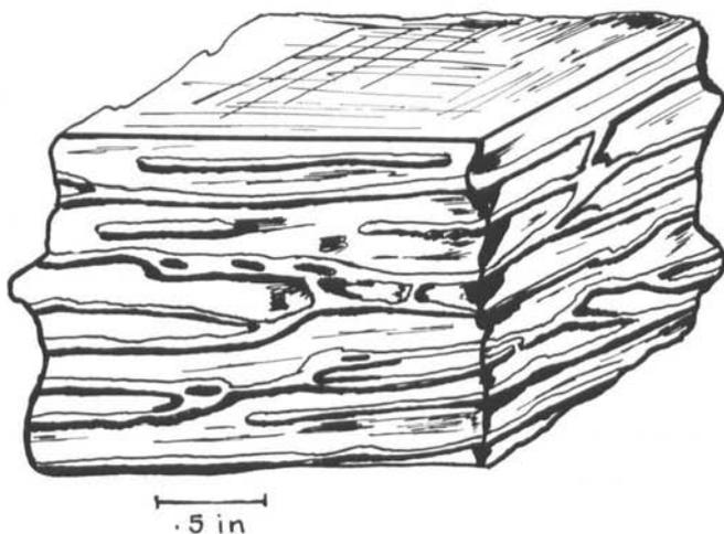
Text-fig. 13. Generalized diagram showing branching and anastomosing, brownish-weathering, silty, raised, dolomitic laminae of typical Crown Point limestone.
