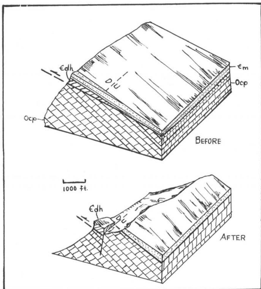
Text-fig. 17. Downfaulted Dunham block west of Champlain Thrust before and after high-angle faulting. Southwest of top of Buck Mt.
