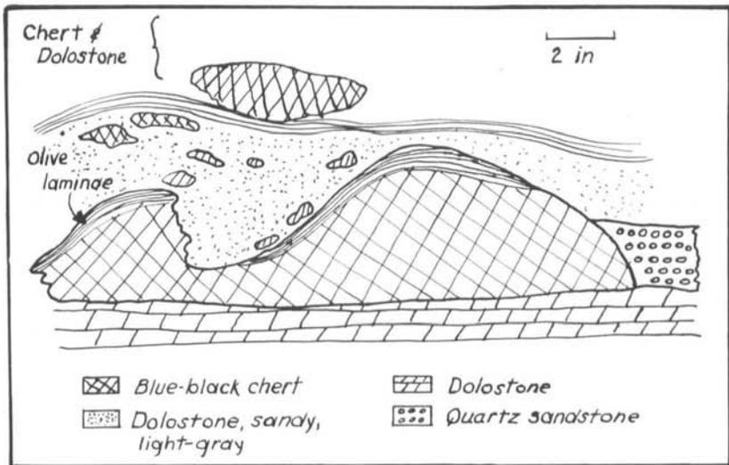
Text-fig. 3. Penecontemporaneous, channeled chert, Ticonderoga dolostone. Smaller fragments of chert are angular and slightly lighter colored than larger chert mass; up to 20%  $\pm$  .75-mm, rounded, frosted quartz grains in sandy dolostone. Location about 30 yards south of bostonite dike which is S. 30° E. of Garden Island, 4 feet above lake level.
