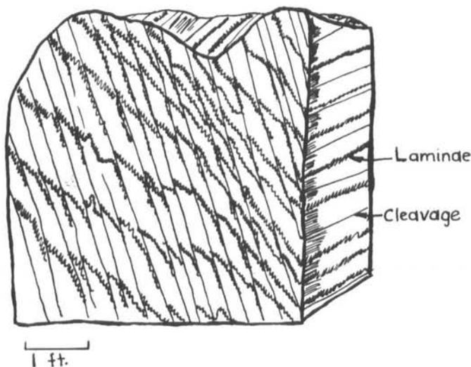
Text-fig. 14. Generalized diagram illustrating cleavage-bedding relationships in Crown Point limestone. Note offsetting of buff- and brownish-weathering laminae along cleavage planes. Generalized from field notes and sketches. See Plate 9, Figure 3 also.
