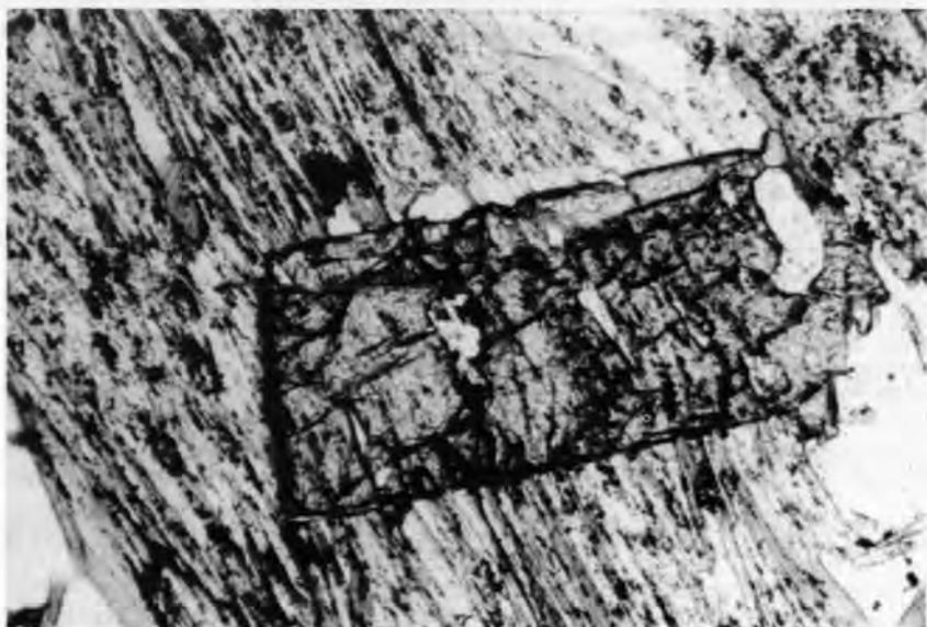
Figure 4-5. Photomicrograph of a staurolite crystal growing across the previously formed schistosity. Sample is from a roadcut in the Northfield Formation on the Green River Rd., 1.5 miles S.72°E. from road junction, Reid Hollow, Halifax. Magnification 40X.
