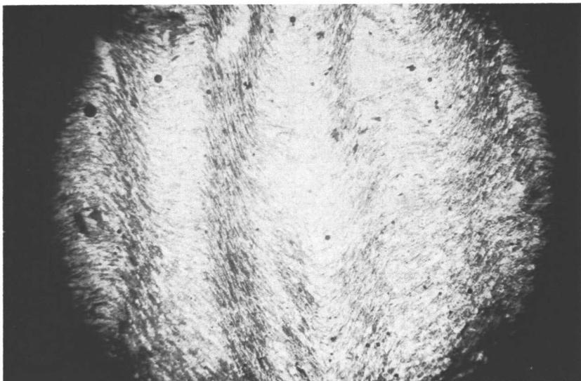
PLATE 33. Photomicrograph showing early stage in development of slip cleavage. Early schistosity is folded and slip cleavage is just beginning to develop. Gile Mountain formation. X12.
