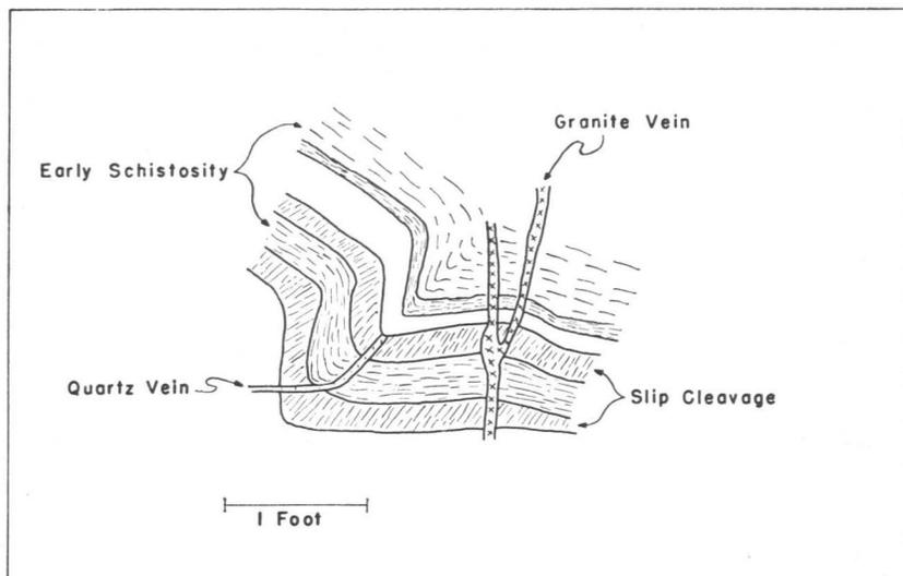
Figure 9. Dextral drag fold of the later deformational stage exhibiting two types of cleavage. Early schistosity and bedding are folded. The later slip cleavage acts as an axial plane cleavage to the fold.
