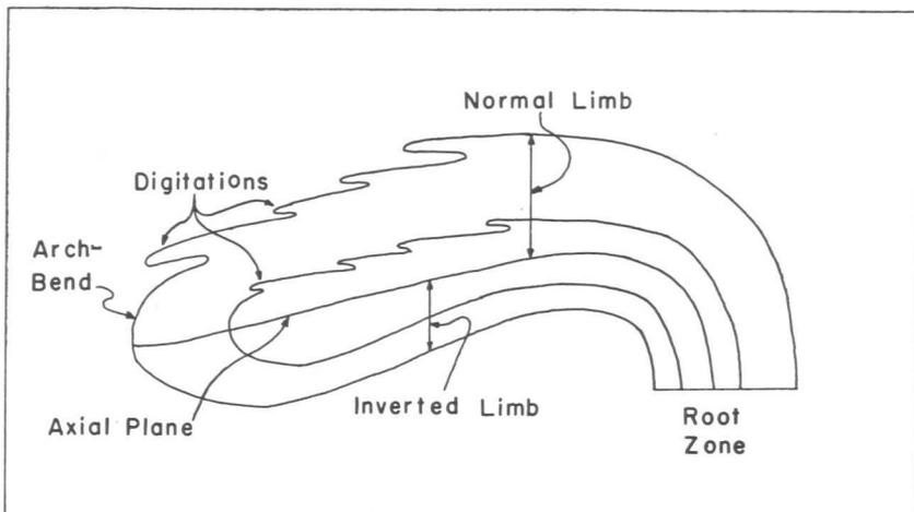
Figure 7. Terminology of parts of a recumbent anticline. Modified from Billings, 1954.
