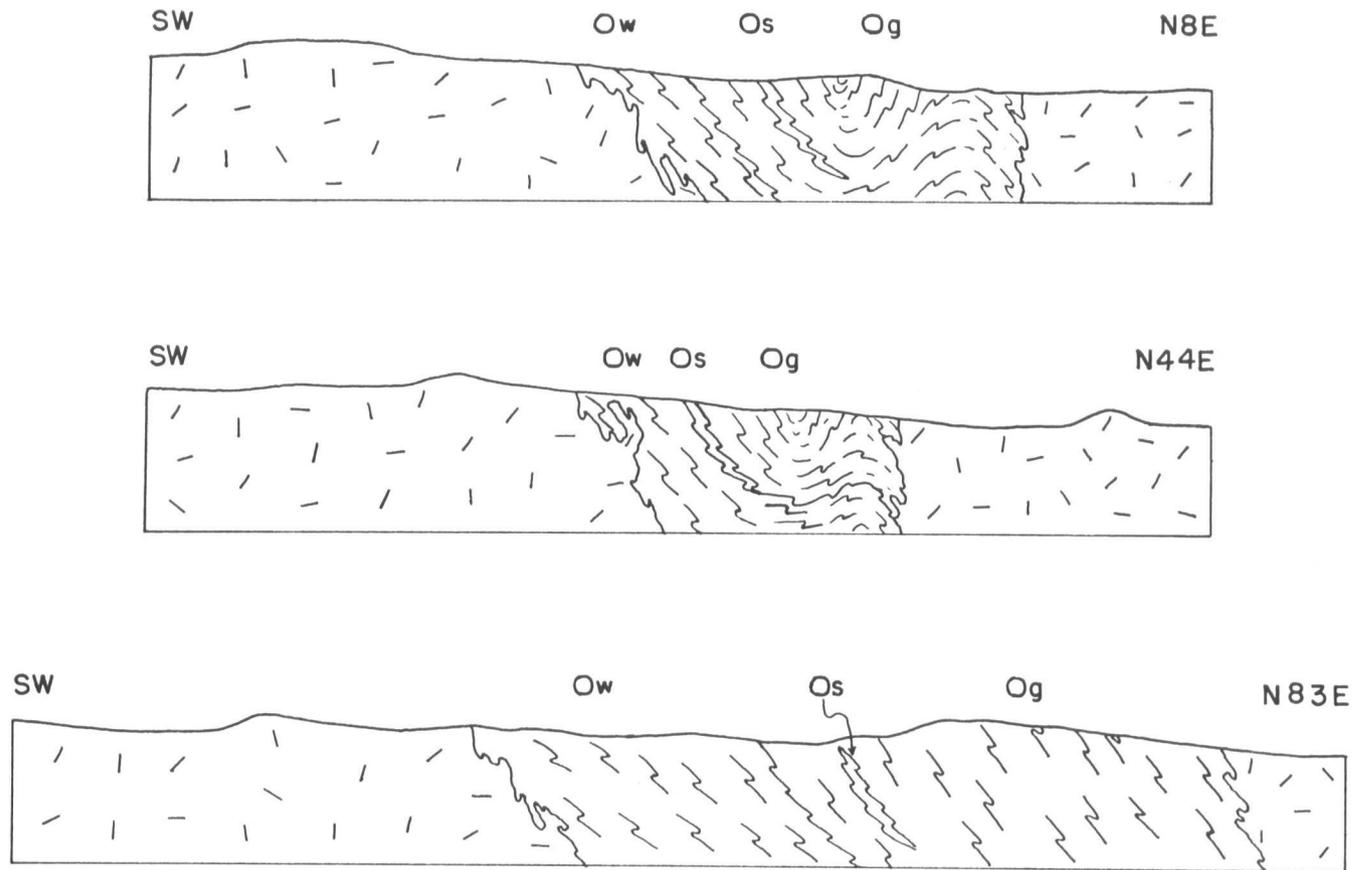
Figure 13. Cross sections radiating northeast in directions indicated from the southwestern corner of the Island Pond quadrangle. Drag folds shown are related to the later deformation. Formation symbols same as on Plate 1.
