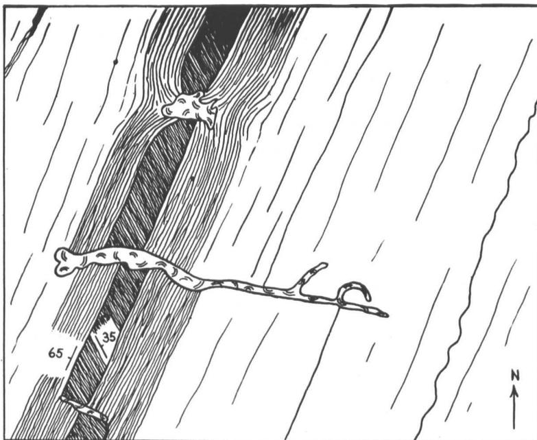
Figure 6. Bed of Barton River between highway and railroad bridge,  $\frac{3}{8}$  mile east of Country Club. Faulted bed of slate and incipient boudinage formation. Barton River formation.
