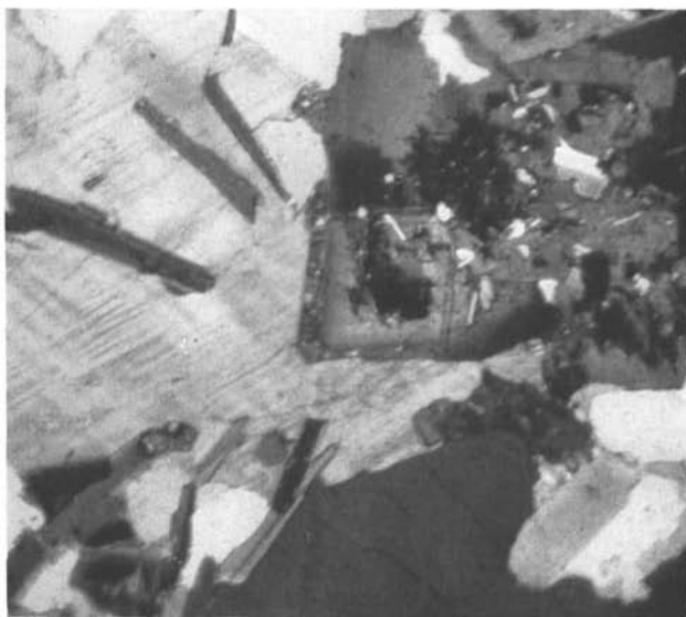
b. Specimen M 59. From disused quarry at D 3030. Microcline, oligoclase, green biotite. Myrmekite at the contact between the zoned oligoclase near the center and the large microcline. Untwinned feldspars are oligoclase.
