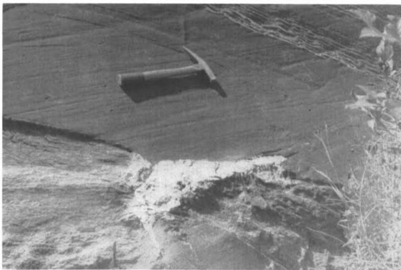
PLATE 11. Boudinage. At G 2752. Competent pelitic schist stretched by flowage in incompetent marble. Quartz has crystallized in the constriction. Quartz-calcite veins delineate the foliation in the marble. Hammer handle is parallel to glacial striations.
