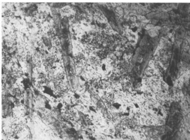
PLATE 18. Standing Pond lava. Below St. Johnsbury dam. Green Laths of hornblende, in groundmass consisting mainly of fine-grained calcic oligoclase.
