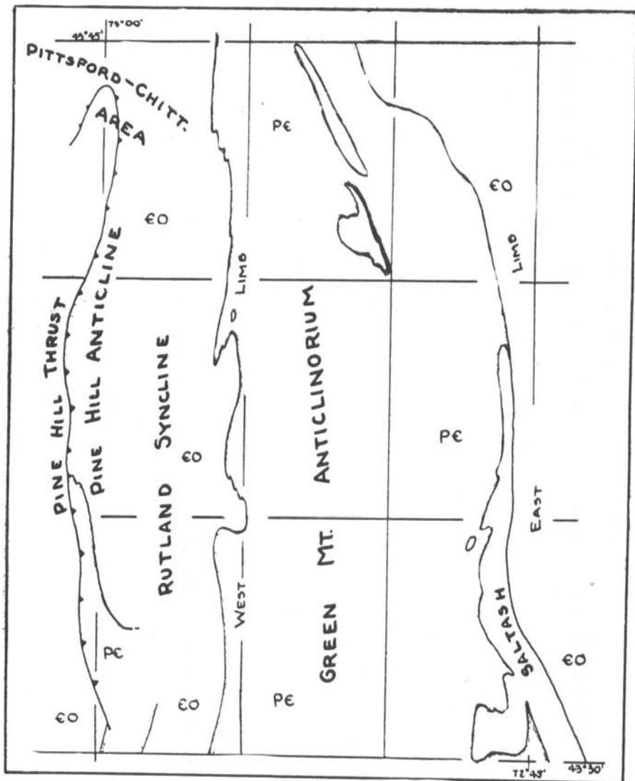
Figure 6. Major Structural Units (sketched from Plate 1, not to scale).
