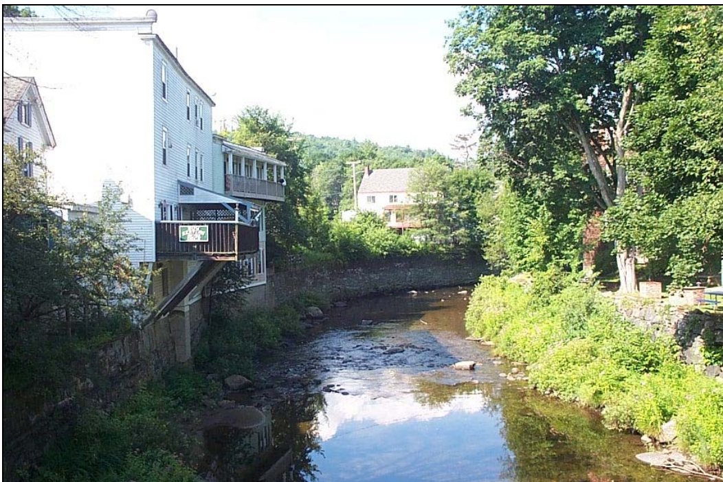
Figure 13: Segment T2.03-A has been extensively channelized through Wilmington village. Historic degradation, widening, and floodplain fill have created a “F” type channel.
