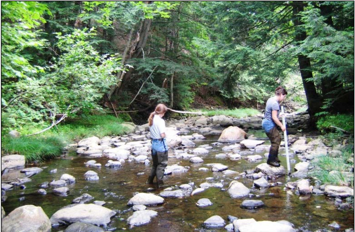
Figure 24: Segment T2.II-A has historically incised and widened into an “F” channel with a plane bed form.
