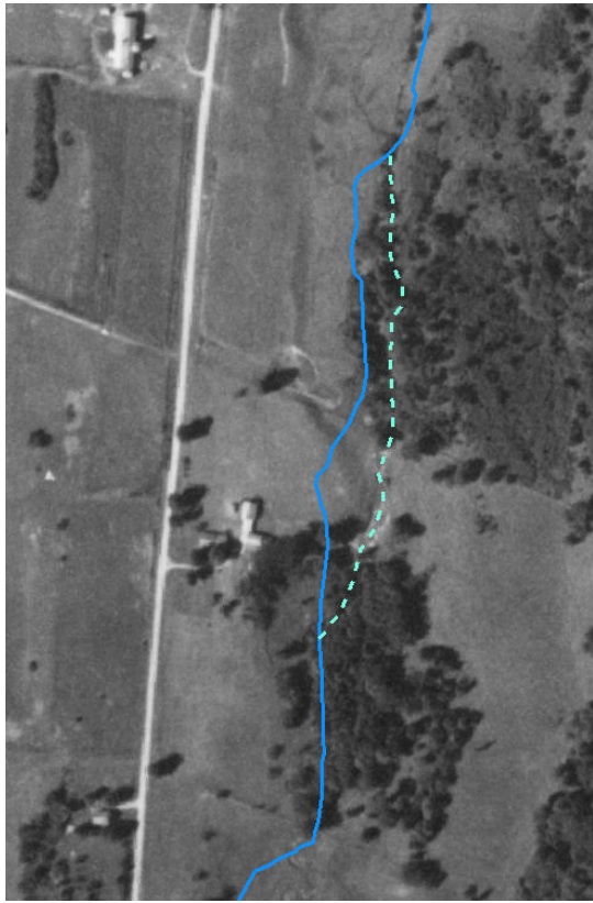
Figure 10 & 11. Aerial photographs of the channel avulsion site from 1937 (left) and 2003 (right). The current channel location is shown in solid blue, and the 1937 channel location in dashed blue.
