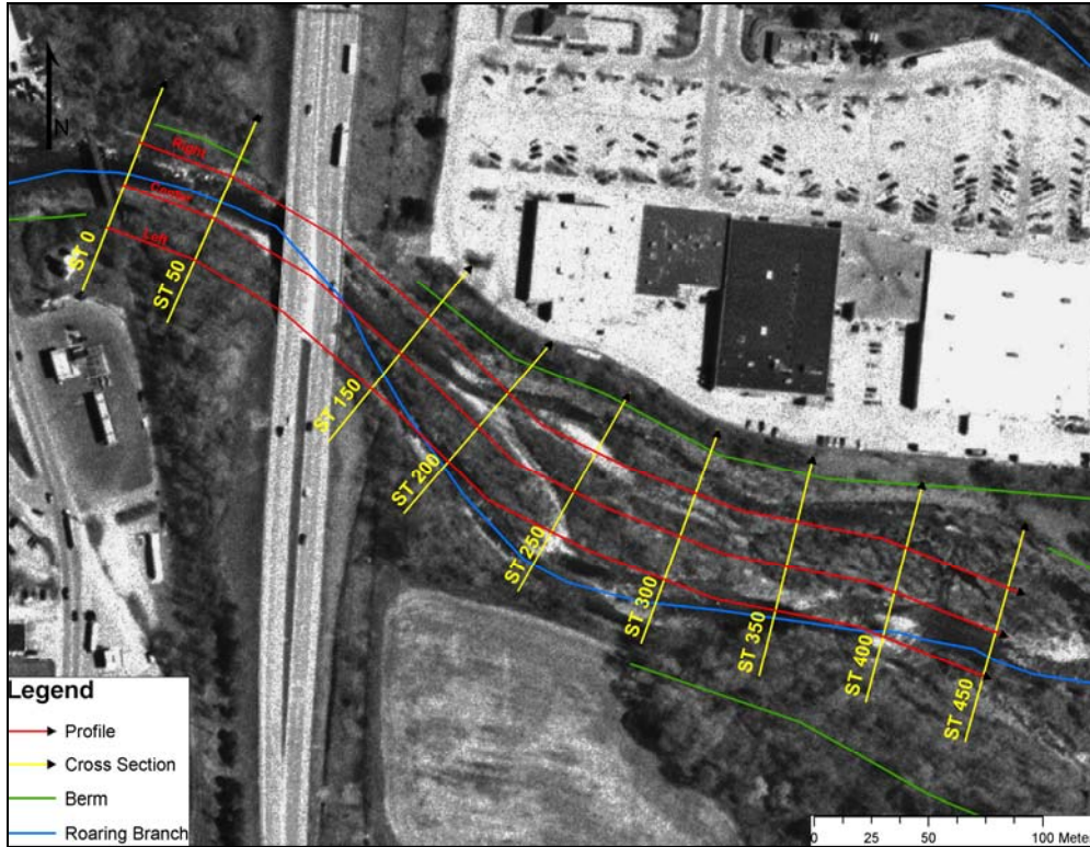
Figure B-31: Route 7 Bridge Sediment Profile and Cross-Section Locations (Orthophoto)
