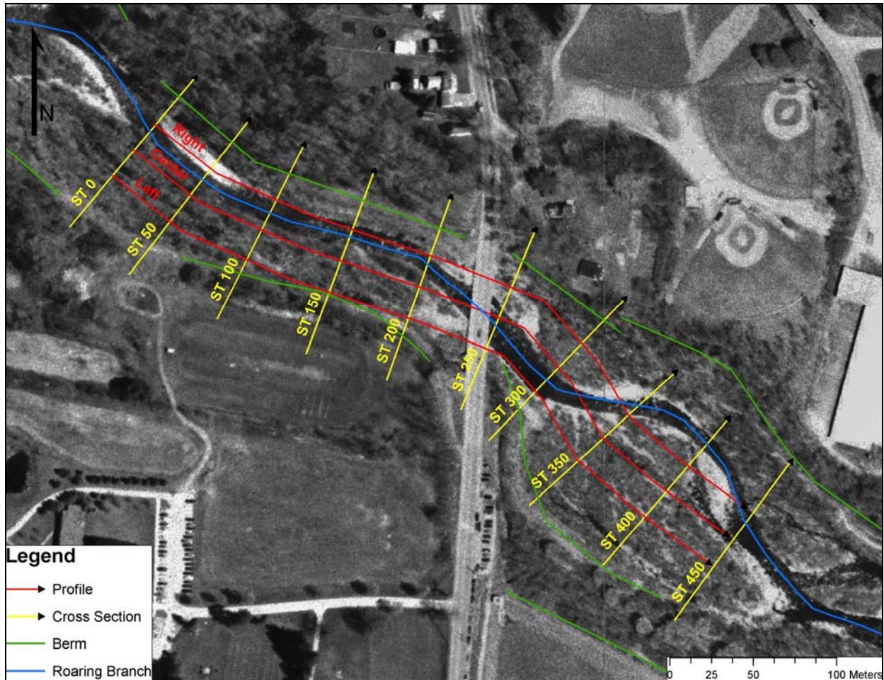
Figure 3-3: Park Street Bridge and Typical Channel Cross-Section.
