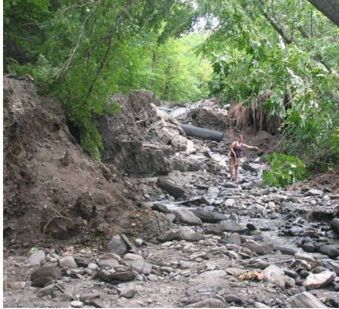
Figure 12. Sediment from a road taken out by this small tributary off of Ayers Brook in Randolph suddenly became a significant contributor to stream dynamics after an intense thunderstorm in July 2007. The woman at center right is indicating the post-flood width of the stream by her armspan.
