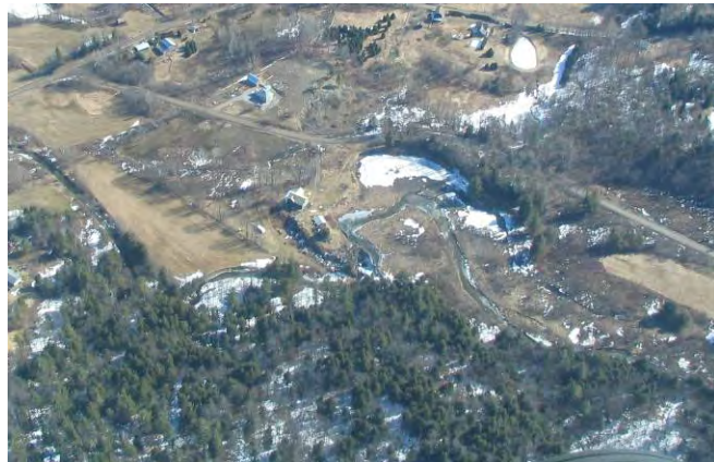
Figure 60. The old mill pond above the Johnson mill dam in Bogue Branch reach T2.05 is now reduced to a mostly single-thread channel, with portions of the old pond (covered in snow here) functioning as an oxbow wetland (2009 aerial photo).
