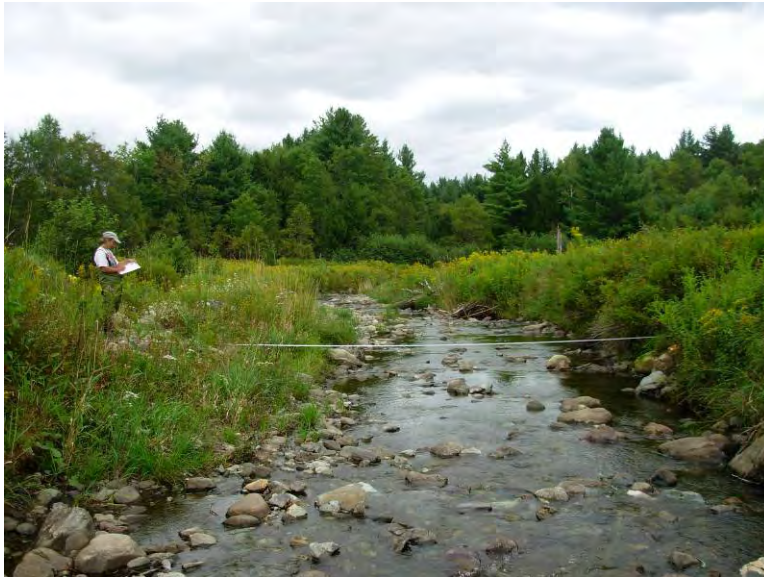
Figure 68: Bogue Branch reach T2S1.03 segment C shows signs of channel straightening and windrowing following beaver damming.
