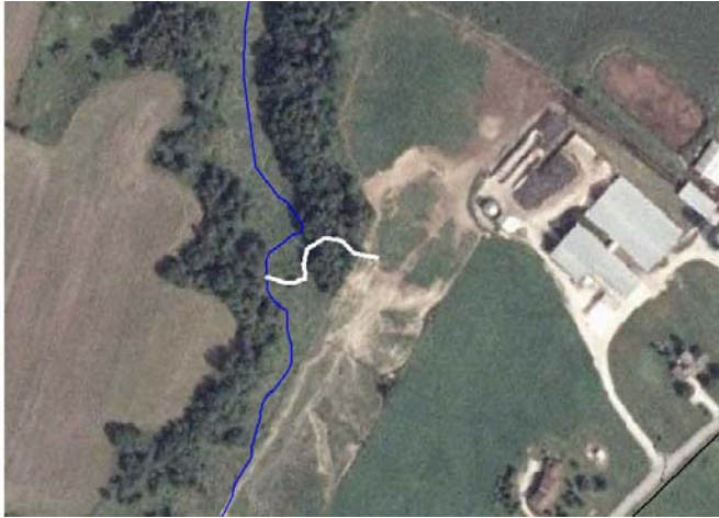
Figure 35. M5S4.01-B. The bold white line at the center of the plan view (left) marks the approximate path of a sediment flow (fine sand and silt) originating in a gully at the margins of the barnyard pasture area (picture right) and leading down the forested valley wall and out into the valley directly to the tributary channel. (Observed on 8 June 2006). Flow in the tributary (blue line) is from south (picture bottom) to north (picture top).
