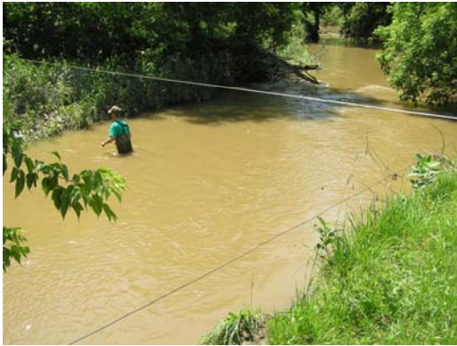
Figure 22. M04. Cross section measurement on 3 July 2006; flows are moderate to high following 30 June and 1 July greater-than-bankfull event; high suspended sediment loads result in very high turbidity.
