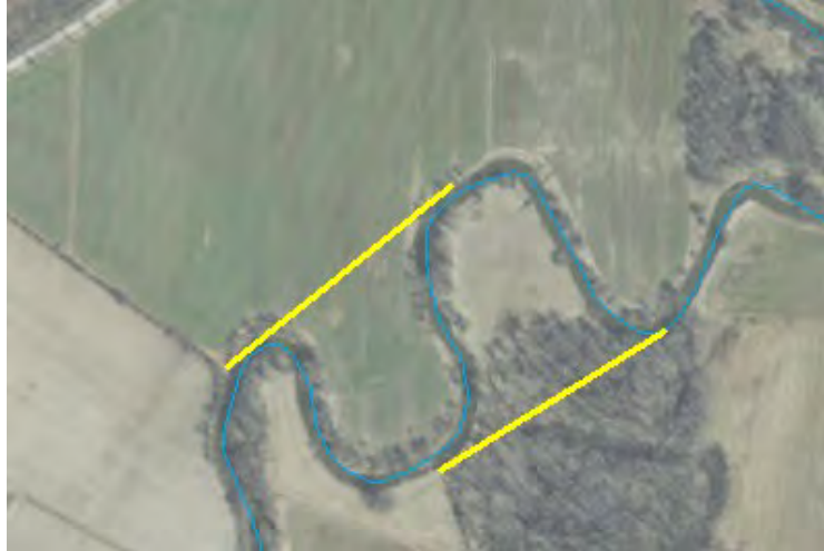
Figure 17: Meander geometry assessment on Reach QM.01
