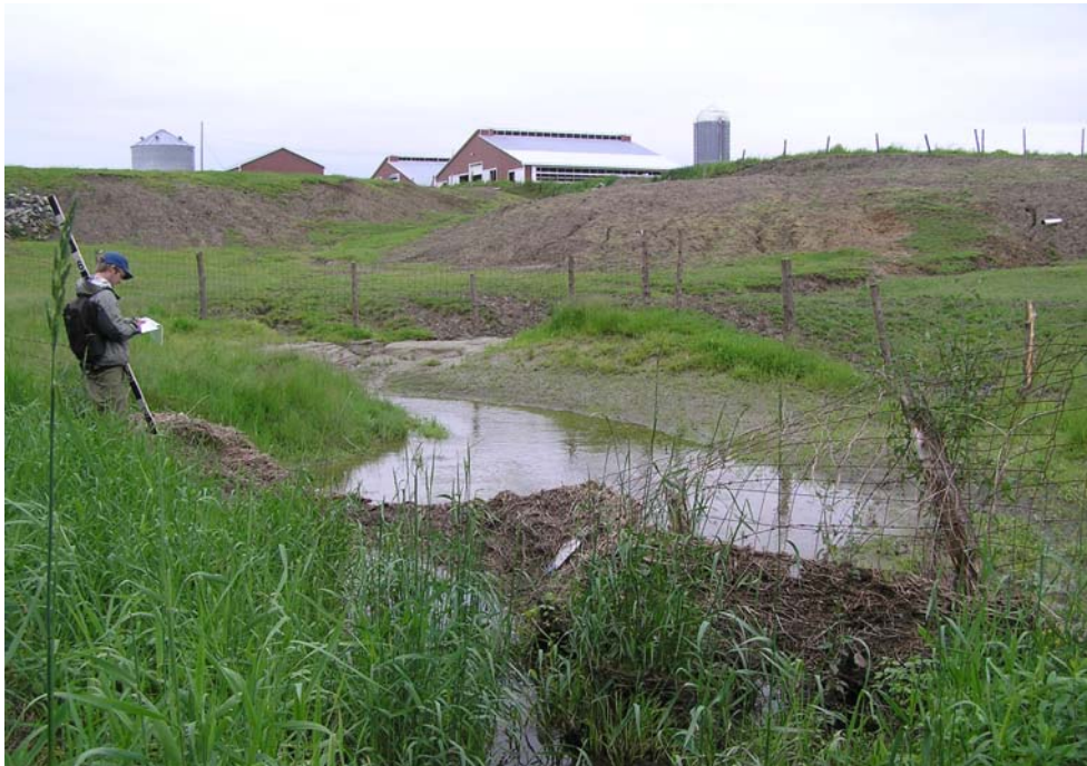
Figure 34. M5S4.01-C. View downstream, 8 June 2006. Debris is caught in a wire fence where a recent avulsion toward right bank has occurred into a high-intensity pasture. Note: Youth Conservation Corps has assisted the landowner in revegetating these slopes as of September 2006.
