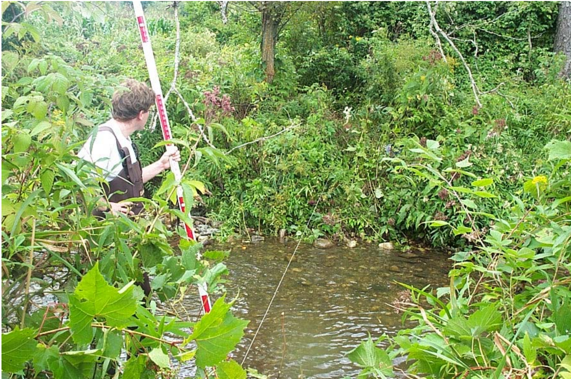
Figure 6. Ben Copans of the Vermont DEC measures the cross-sectional area of the Upper West Branch during summer 2005.
