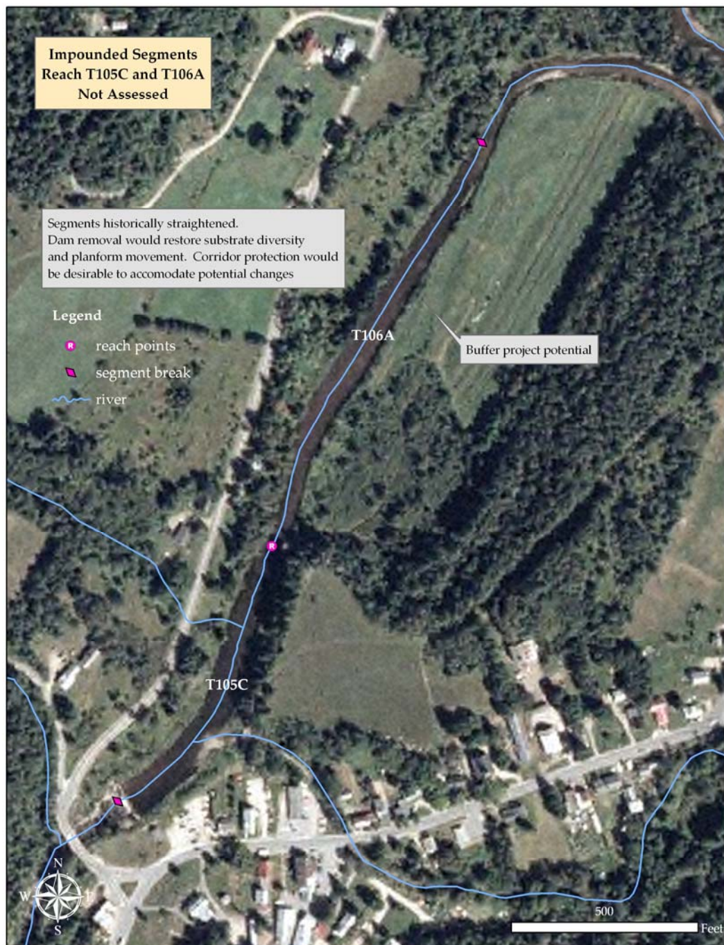
Figure 37: Impounded segments upstream of East Burke Dam
