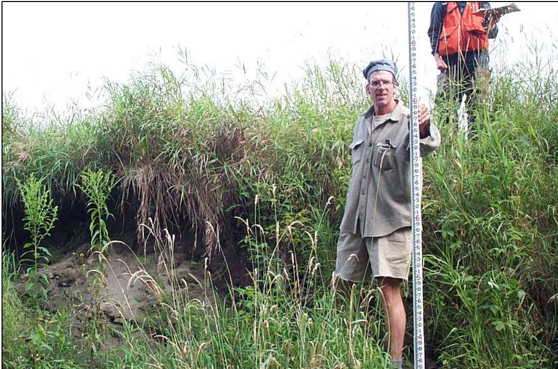
Figure 5. Charlie Wanzer, high school science teacher in Cabot holds the rod to measure the bank height. The low bank height within this segment was close approximately 8 feet, providing evidence that the Winooski is incised in this location.
