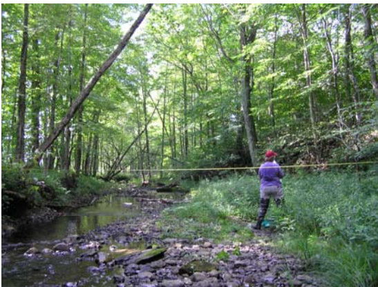
Figure 36. In Segment T02.09-s1.04-E, North Bretton Brook is incised ( IR= 2.2 ) between the bedrock-controlled right valley wall and corn fields along left bank. View downstream, 2 August 2005
