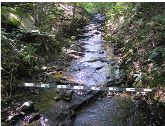
Figure 43. T02.08-s1.05-E A1-cascade bedrock channel flows through a deciduous forest to the west of Pond Hill Ranch Road. View upstream, 25 July 2006. River staff is at approximate bankfull elevation.
