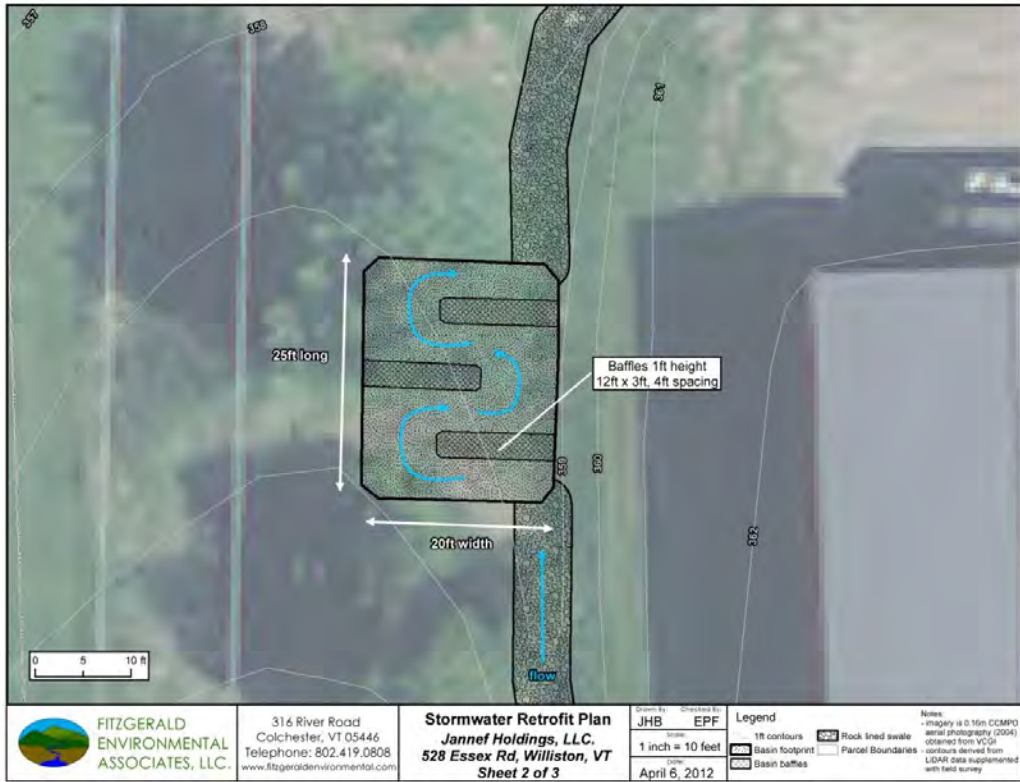
Figure 22: Example of baffled sediment basin.
