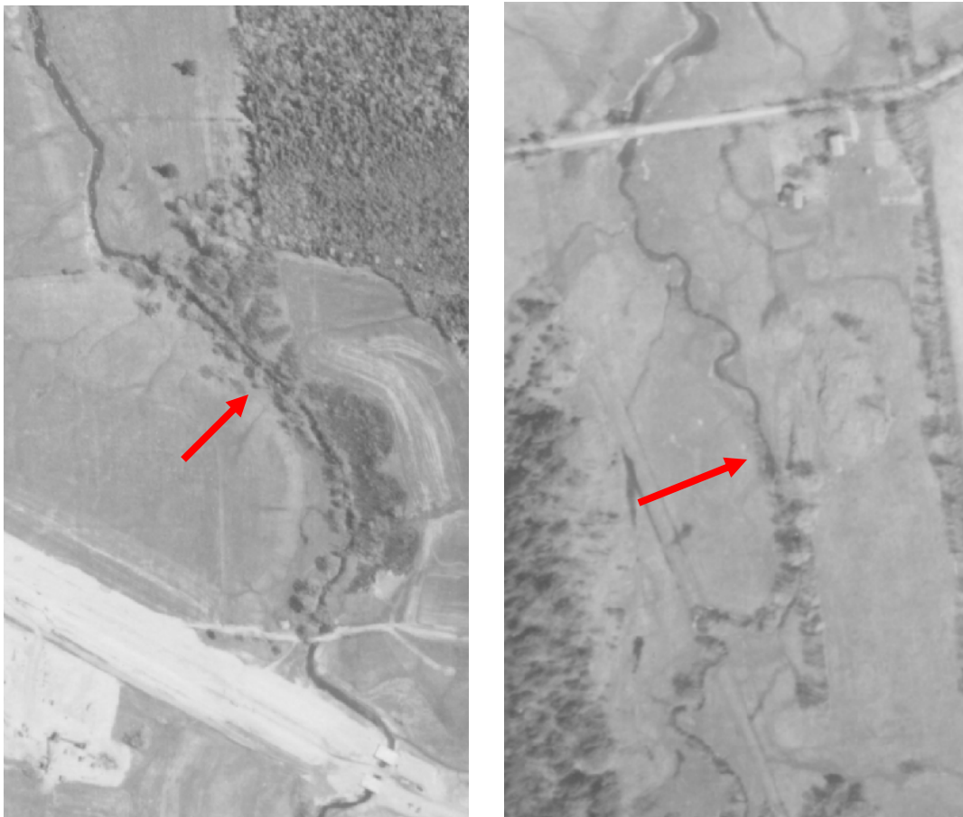
Figure 9. Historical channel straightening north of I-89 (left) and south of Van Sicklen Road (right) as seen in aerial photography from 1962.
