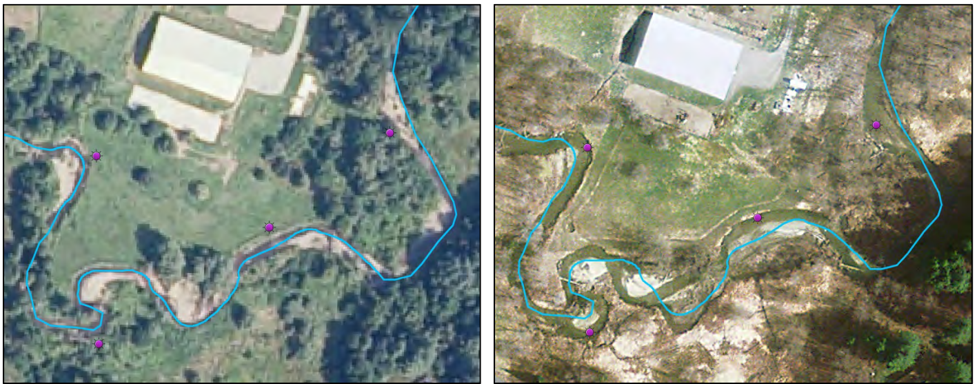
Figure 1. Side by side comparison of a location along Thatcher Brook where meander migration (purple dots) occurred likely as a result of TSI (2009 imagery on left, 2013 on right).
