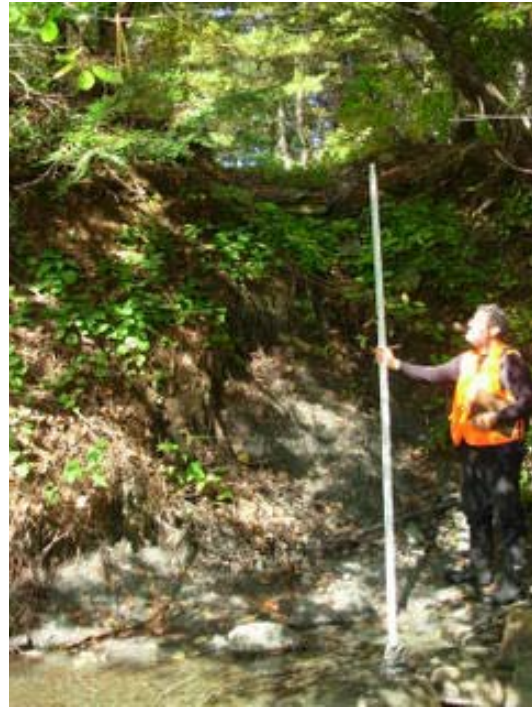
Figure 33. Norwich Conservation Commission volunteer Jonathan Frishtick extends a measuring rod near bank erosion located just above a headcut in the stream.
